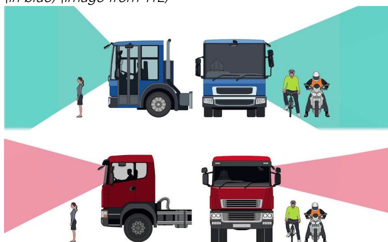
Comparison of direct vision coverage between conventional (in red) and Direct Vision HGV (in blue) (image from TfL) 49
