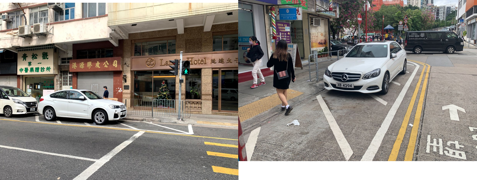
Figure 50 & 51: Painted hatched marking are ineffective in deterring parking that obstructs pedestrian sightlines
