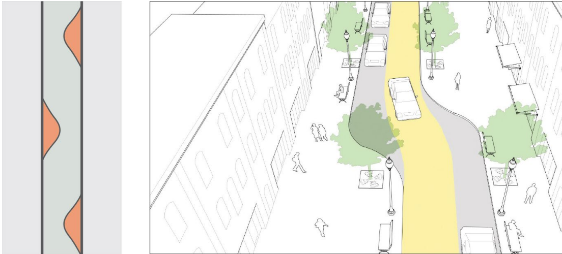
Figure 44: A chicane used in Singapore's Silver Zone (image from LTA) 62
