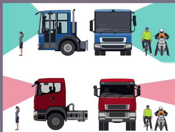
Figure 58: Comparison of direct vision coverage between conventional (in red) and Direct Vision HGV (in blue) (image from TfL) 70
