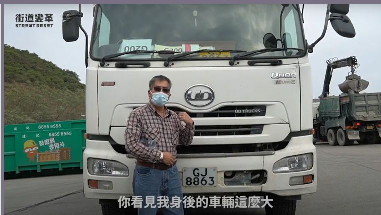
Figure 57: Large vehicle size makes it difficult for drivers to detect pedestrians if they are within 3 metres of the front of the vehicle. Note that the vehicle shown is classed as a medium goods vehicle.
