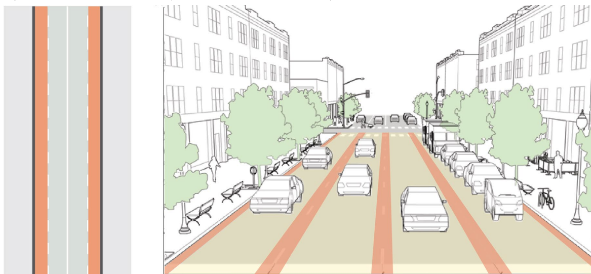
Figure 40: Lane width reduction (illustration adapted from GCDI) 57
